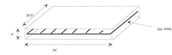
Specifications: Concrete minimum strength 4500 psi at 28 days Air entrainment- minimum 5 % Reinforcement- Gal. WWM Finish- Edged and broomed
