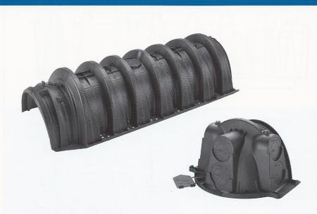
The evolutionary patent-pending Quick4® Equalizer® 36 Chamber fits in a 24" wide trench and is ideal for curved or straight systems. It features the patent-pending Contour Swivel Connection™ which permits 15-degree turns, right or left. The MultiPort™ end cap allows multiple piping options and eliminates pipe fittings. The chamber's four-foot length provides optimal installation flexibility.
