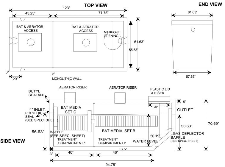
Specifications: Concrete minimum strength-5000 psi at 28 days
