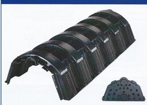
The High Capacity Infiltrator Chamber H-20 offers maximum internal volume per linear foot for extra temporary storage capacity. The 10" louvered sidewalls facilitate infiltration and evapotransporation, while reducing fines in the system. The High Capacity H-20 chamber gets an H-20 load rating with 18" of compacted cover when installed per installation requirements.
