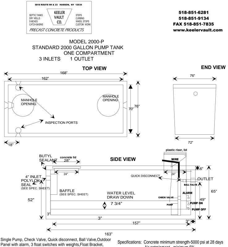
Weep hole,SS Wire Rope DRAW DOWN IS 45.65 GALLONS/INCH Draw down should not not be less than 4" due to float design.
