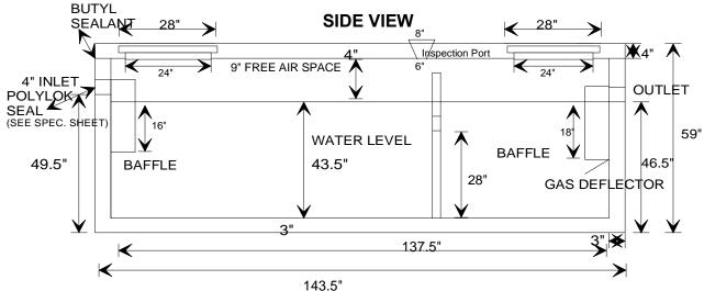
Specifications: Concrete minimum strength-5000 psi at 28 days
