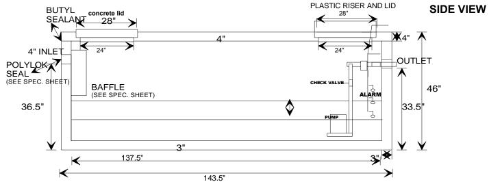
Specifications: Concrete minimum strength-5000 psi at 28 days
